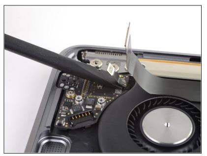
Slide the flat end of a spudger underneath the Touch ID sensor cable to slice through the adhesive securing it to the audio board.
