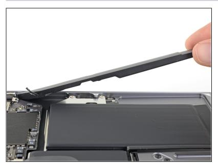
• Lift the left speaker straight up from the bottom and remove it.
