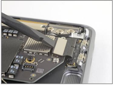
Use the flat end of a spudger to pry the USB-C cable connector up and out of its socket on the logic board.
