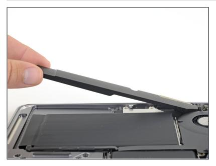
Lift the right speaker straight up from the bottom and remove it.
