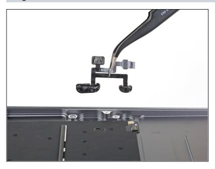
Remove the microphone assembly.
