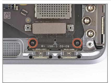
Use a T4 Torx driver to remove the two 2.9 mm screws securing the USB-C board.
