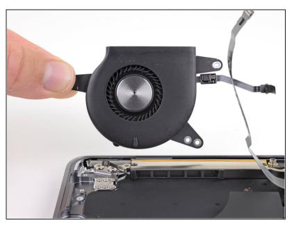
• Lift the fan out of the case and remove it.
