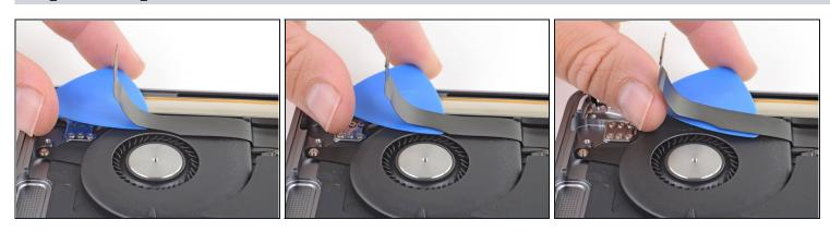
Slide an opening pick under the audio board cable to slice through the adhesive securing it to the fan.
