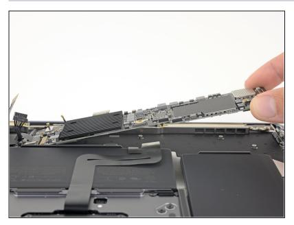
• Remove the logic board.
