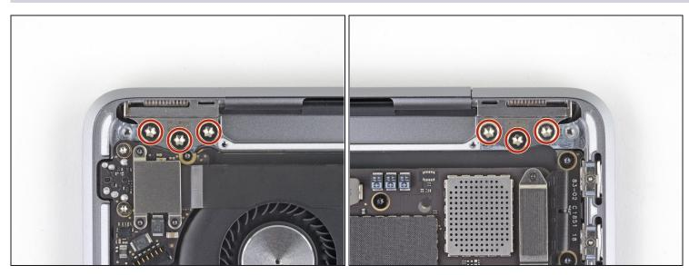
• Use a T9 Torx driver to remove the six 4.9 mm screws securing the display hinges to the upper case.
