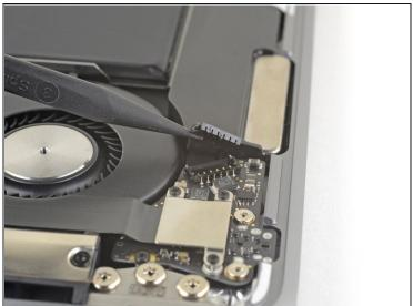
Slide the tip of a spudger underneath the speaker cable and pry straight up to disconnect the speaker.
