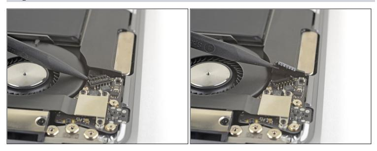
• Slide the tip of a spudger underneath the right speaker cable and pry straight up to disconnect the speaker.
