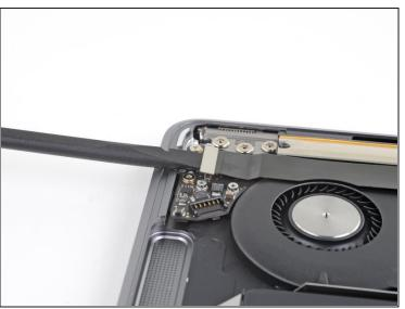
• Use the flat end of a spudger to pry the audio board connector straight up and disconnect it.
