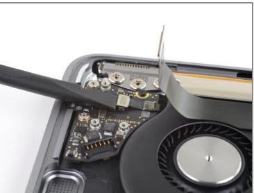
• Use the flat end of a spudger to pry the Touch ID sensor connector straight up and disconnect it.
