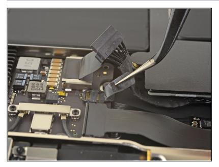
Peel back the black tape covering the fan cable connector.
