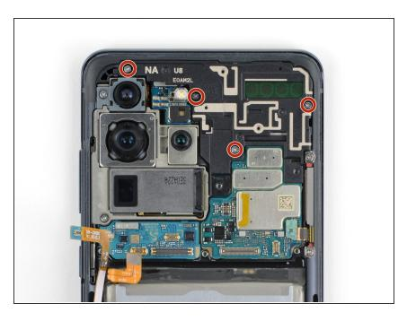
Use a Phillips #00 screwdriver to remove the four 3.9 mm-long screws securing the upper midframe.
