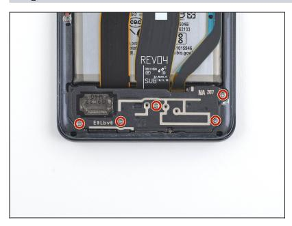
Use a Phillips #00 screwdriver to remove the five 3.9 mm-long screws securing the loudspeaker and lower midframe.
