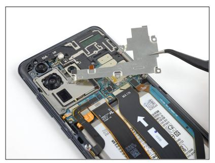
Use a pair of <u>tweezers</u> to unclip and remove the motherboard bracket.
