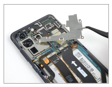
• Use a pair of tweezers to unclip and remove the motherboard bracket.
