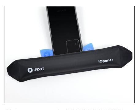
Apply a heated iOpener to the top edge of the back cover for two minutes.
