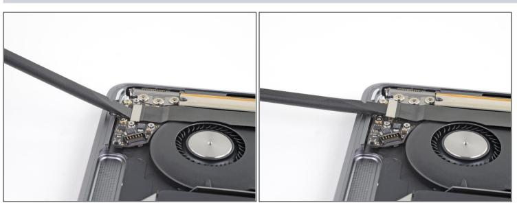
• Use the flat end of a spudger to pry the audio board connector straight up and disconnect it.
