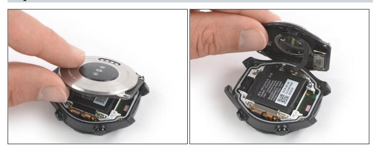
Carefully fold the back cover assembly to the opposite side of the two watch crowns.
