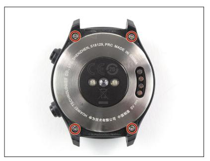
• Remove the four Torx T2 screws (4.5 mm length).
