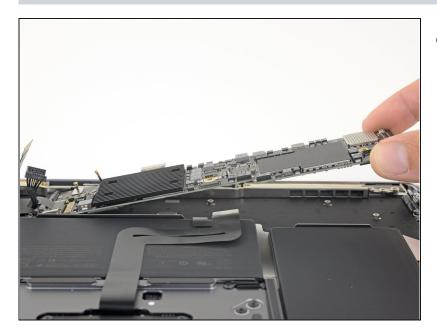
Remove the logic board.
