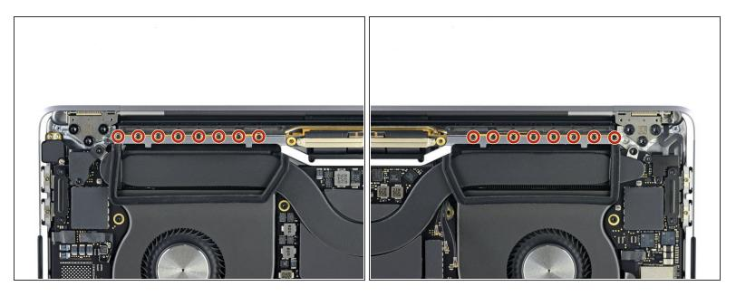
Use a P2 Pentalobe driver to remove the sixteen 1.5 mm screws securing the antenna assembly (eight on each side).
