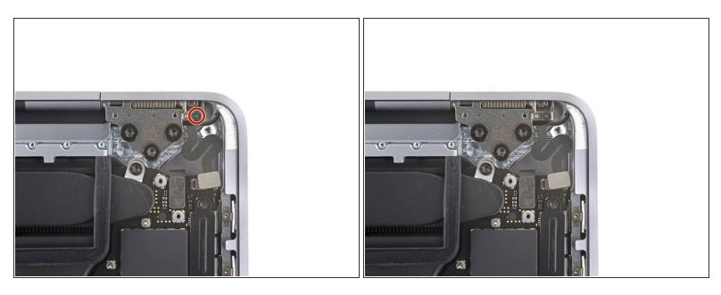
Use a P2 Pentalobe driver to remove the 1.9 mm-long screw securing the lid angle sensor.
