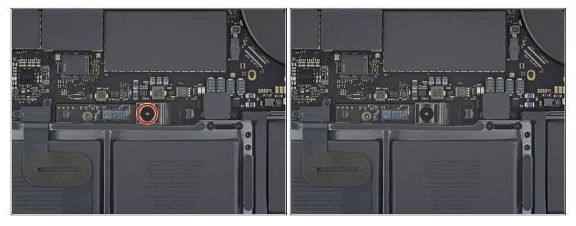
• Use a T5 Torx driver to remove the 6.7 mm pancake screw securing the battery power connector.
