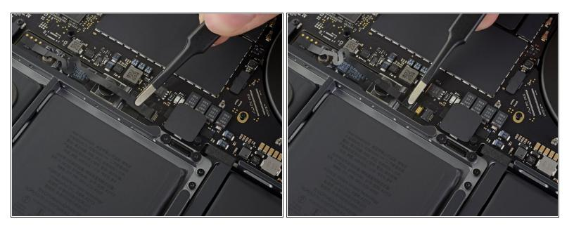
Disconnect the battery board data cable by sliding it out from its socket on the logic board.
