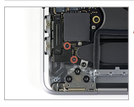
Using a T3 Torx driver, remove the two 1.5 mm screws securing the cover bracket for the Touch Bar digitizer and lid angle sensor connectors.
