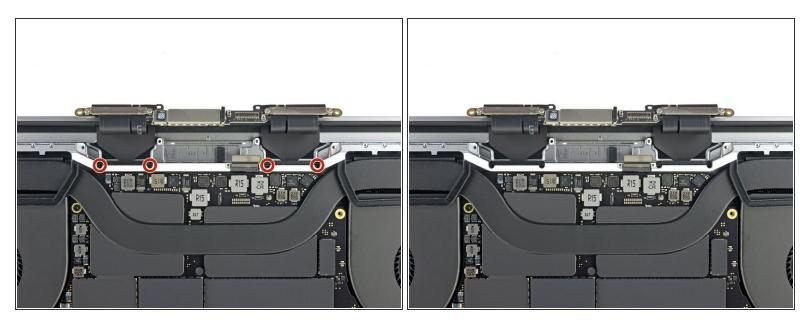
• Use a T3 Torx driver to remove the four 3.9 mm screws securing the display cable cover springs.
