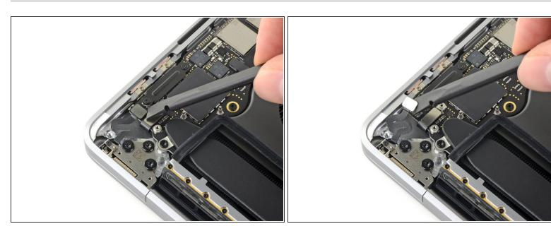
Disconnect the lid angle sensor cable by prying it straight up from the logic board.
