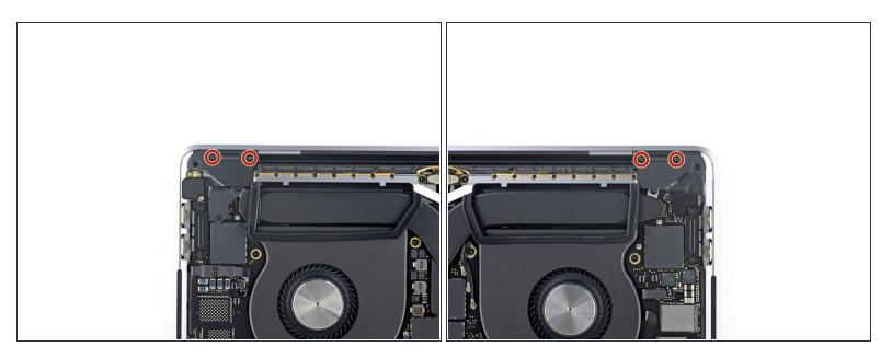
Use a T3 Torx driver to remove the four 2.0 mm screws from the hinge covers (two screws on each side).
