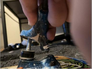
To reassemble, take the lower cup washer, then the lower bushing and put it on the kingpin. Next, set the replacement hanger on top of the lower bushing.
