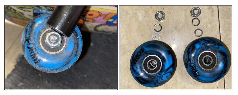
Using the T-tool, unscrew the nut securing the wheel and remove it, setting it and the wheel aside.
