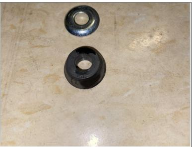
Pull straight up to remove the hanger. Remove the lower bushing and the lower cup washer just to check on the riser.
