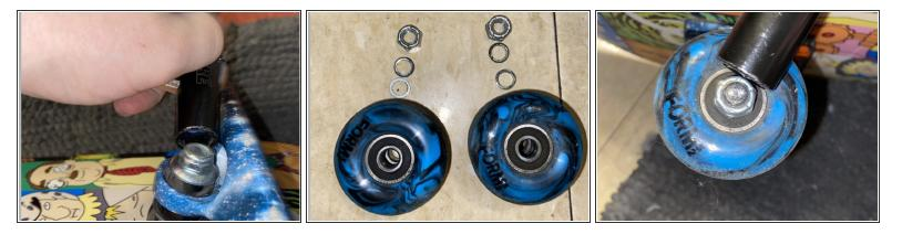
After the kingpin nut is secured, take your T-Tool and add the wheels back onto and secure them in place.
