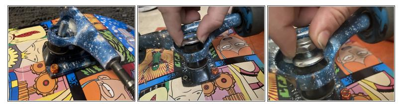
After the hanger is added, put the top bushing, the top cup washer and then the Kingpin nut back.
