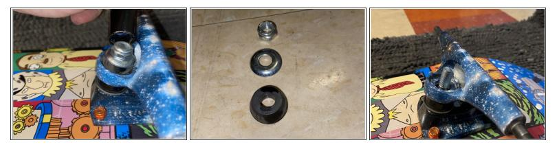
Using the T-Tool, unscrew the Kingpin nut, washer and top bushing so that the hanger itself can be taken off.
