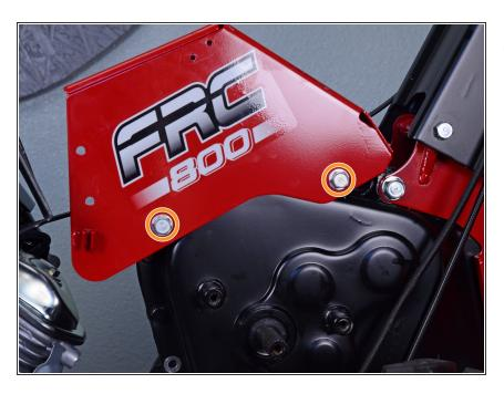
Use a 14 mm socket to remove the two shift gate through-bolts.
