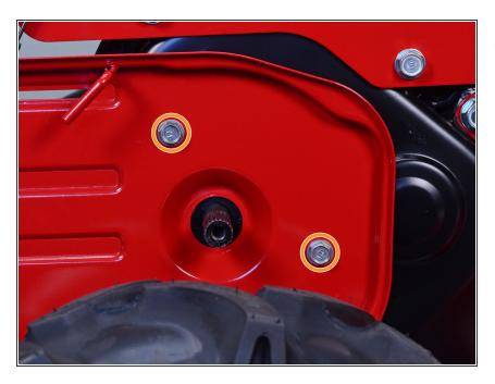
Use a 12 mm socket to remove the two remaining inner belt cover bolts behind the transmission pulley.
