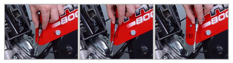
Pull up on the clutch cable to remove it from its slot.
