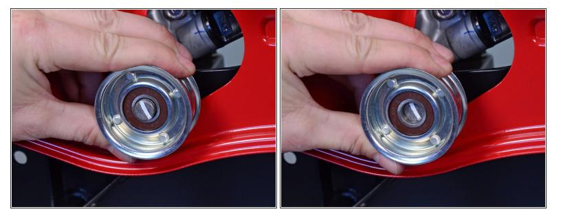
Remove the tensioner pulley.
