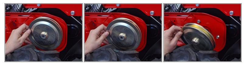
Pull the transmission pulley straight off of the splined shaft to remove.
