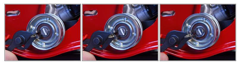
Use snap ring pliers to remove the snap ring securing the tensioner pulley to its shaft.
