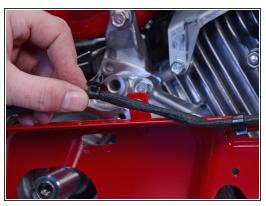
Use needle nose pliers to remove the three wire clips securing various cables to the back of the inner belt cover.
