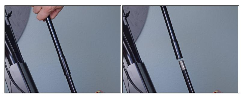
Slide the change lever extension off its base to remove.
