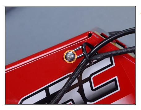
Use a Phillips #1 screwdriver to remove the cable guide screw.
