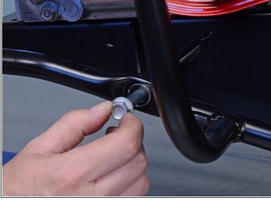
Remove the frontmost guard bolt.
