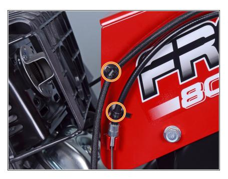
Use needle nose pliers to <u>remove</u> the cable clips.
