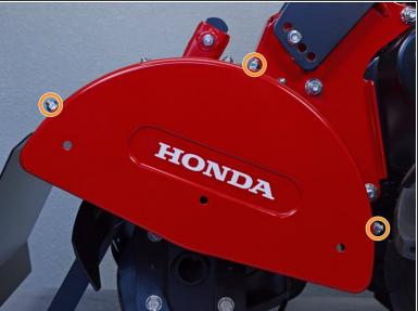
Use a 12 mm socket and wrench to remove the six sets of side guard bolts and nuts, three on each side.
