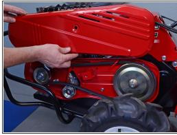
• Tilt the outer belt cover down and pull it off of the lip on the inner belt cover to remove it.
