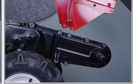
Rotate the blade guard up and off of the transmission to remove it.
