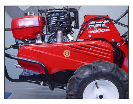
Use a 14 mm socket to remove the bolt securing the outer belt cover.
