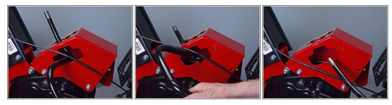
Pivot the shift lever out and away from the shift gate to remove it.
