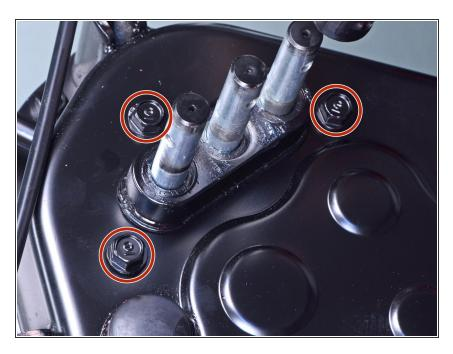
Use a 12 mm socket to remove the three bolts securing the shift holder to the right transmission case.
