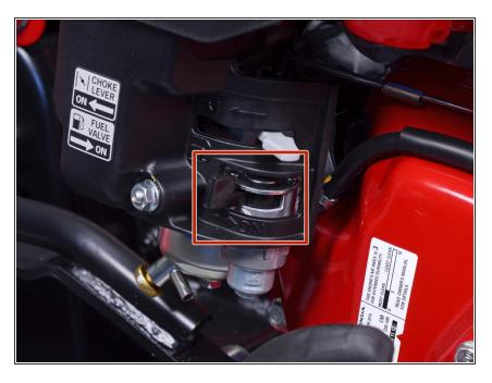
Flip the fuel valve switch to the off position.
