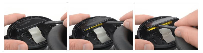
Insert the flat end of a spudger between the battery cover and the battery.
