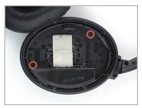
Remove the two Phillips #00 screws (6.2 mm length).
