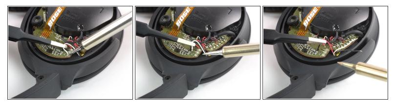
Use a soldering iron to desolder the three battery cables from the circuitboard.
