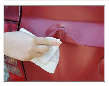
Wipe down the area of the paint chip or scratch with a damp papertowel.
