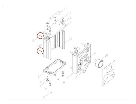
Remove the back cover, fixed by four screws.
