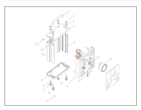
Remove the manometer by unscrewing the two retaining nuts.
