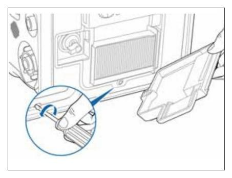
To access the HEPA filter, first remove the screw holding the filter cover in place and gently remove the cover.
