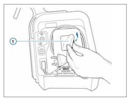
The fan filter is located on the side of the ventilator and can be removed and replaced by hand.
