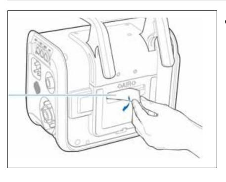
The air intake filter is located on the rear of the device, and can also be removed by hand.
