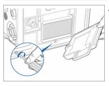
Remove the screw in the bottom center of the panel, and then take the panel off.
