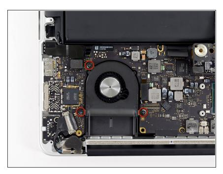
Remove the three 3.1 mm T5 Torx screws securing the left fan to the logic board assembly.
