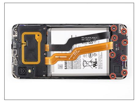
Remove the 8 Phillips #00 screws on the bottom (3 mm length).
