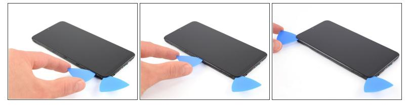
Insert a second opening pick and slide it to the top left corner. Leave the opening picks in place to prevent the adhesive from resealing.
