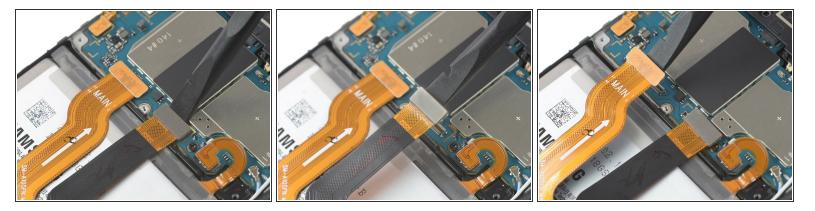
Use the flat end of a spudger to pry up and disconnect the display flex cable from the motherboard.
