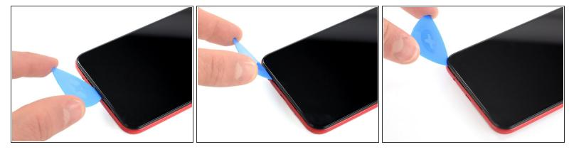
Slide the opening pick to the bottom left corner to release the clips.
