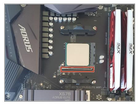
Remove the CPU from the motherboard by raising the retention arm. Lay the CPU carefully on a soft surface to avoid damaging him by deforming some pins.
