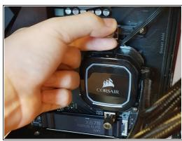
Reattach the screws that connect the CPU cooler and wires to the motherboard.
