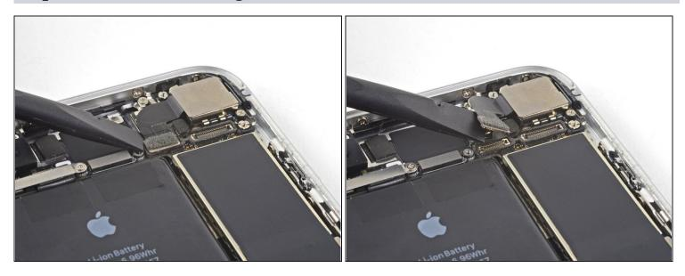
• Use the flat end of a spudger to disconnect the camera cable connector by prying it straight up from its socket.
