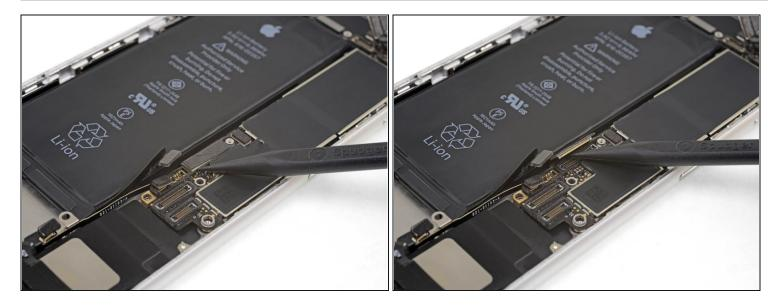
• Use the point of a spudger to pry up and disconnect the Lightning cable connector.
