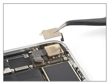
• Remove the rear-facing camera bracket.
