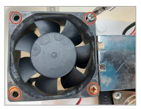
Secure the new fan with the four 30 mm screws using a Phillips #2 screwdriver.
