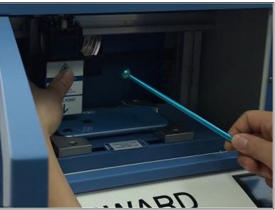
We put the whole phone into Blue Light Laser Separation Machine to laser the back glass so that we can easily remove the back glass, by then.
