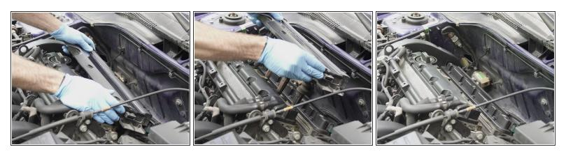
Grip the ignition coil pack on both sides and pull it directly upwards to remove it.
