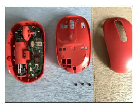
I unscrewed the 3 Torx T6 Screws holding the body onto the bottom case
