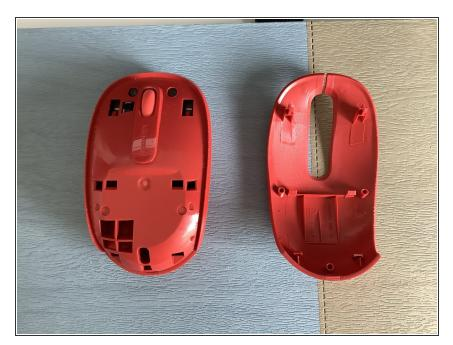
I unclipped the 9 clips holding the top case to the body.
