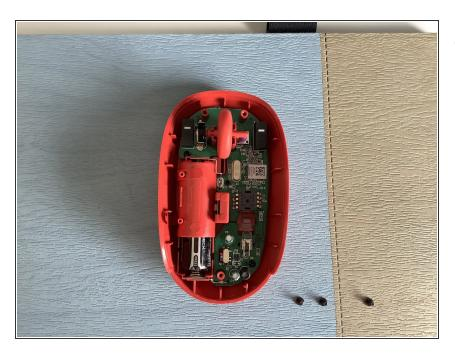
I undid the two Philips #00 screws on the motherboard
