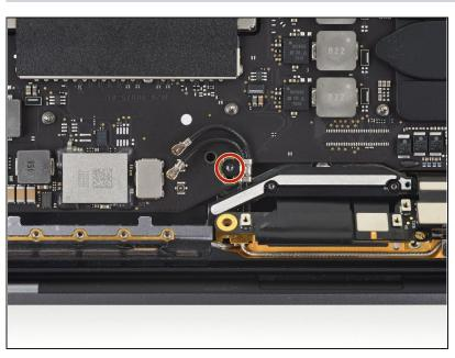
Remove the 2.8 mm T5 Torx screw securing the two antenna coax cables to the main board.
