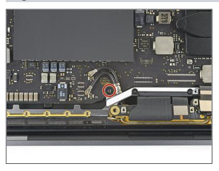
Remove the 3.4 mm T5 Torx screw securing the two antenna coax cables to the main board.
