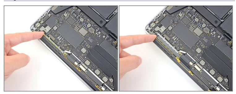
• Carefully remove the antenna assembly while simultaneously feeding the antenna cable bundle out from underneath the heat pipe.
