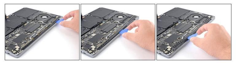
• Use an opening pick to lever out the antenna cable assembly in the areas shown.
