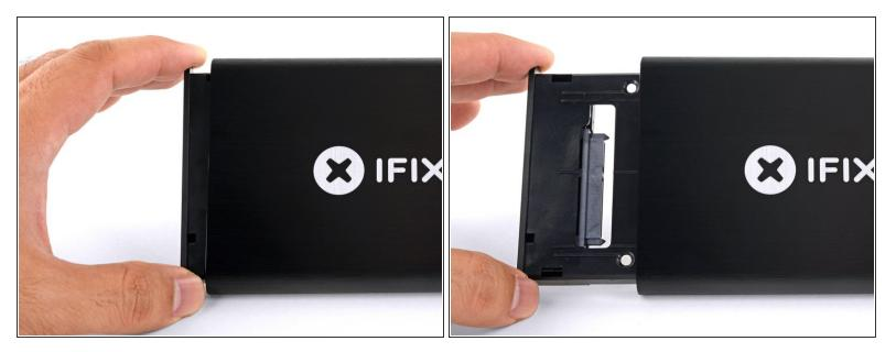
Slide the plastic tray out of the aluminum housing.
