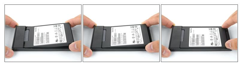
• Set the drive in the plastic tray and align the drive ports with the tray socket.
