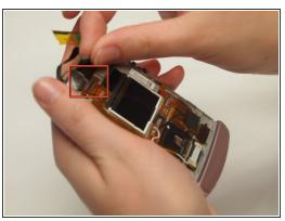
Detach the ribbon connections underneath the green connector strip and remove them from the device. This will reveal the camera.
