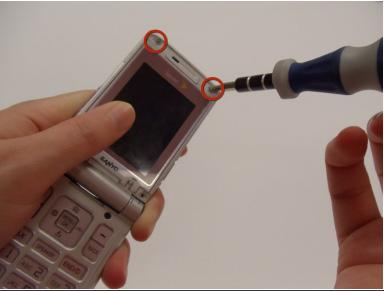
Remove the 4.4mm screw in each corner using the Tri-wing Y0 screwdriver.
