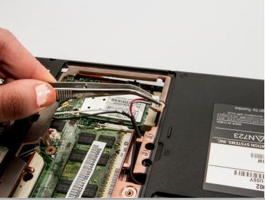
Grasp the power cable with your tweezers and remove it from the wireless antenna.
