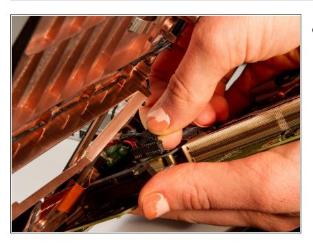
Lift the back panel and carefully disconnect the main power cable.
