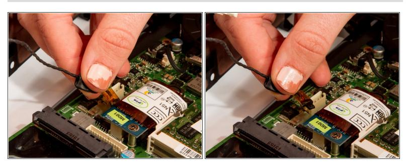
Remove the black signal cable attached at the blue circuit board.
