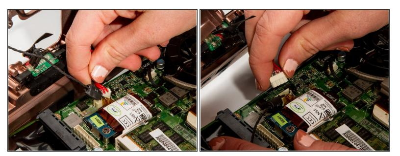
Remove auxiliary power cable attached to the blue board at the back of the laptop.
