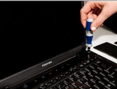
Using #1 Phillips Screwdriver, remove both of the 5 mm screws that are located beneath the insert.
