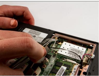
Locate and remove both the white and black antenna leads with the tweezers.
