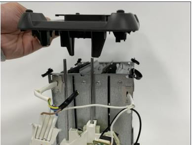
Once the wires have been completely pulled out of the toaster the base can then be removed from the middle component.
