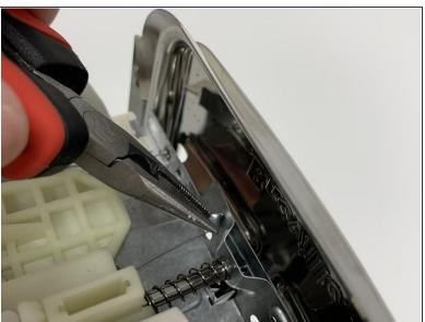
Same applied here, using pliers pull out the tabs.
