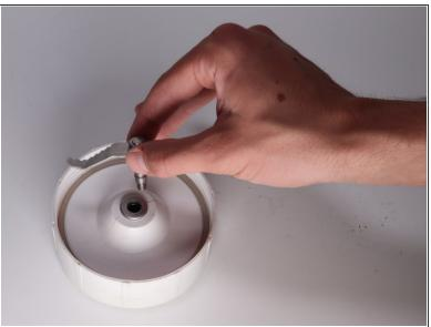
Now that all the fixtures are removed the blade can be lifted out of the housing.
