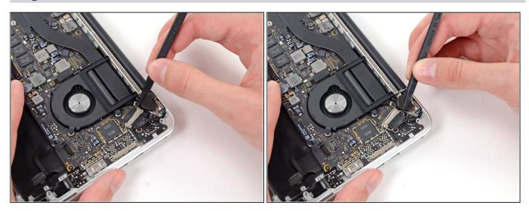
• Use the tip of a spudger to rotate the pull tab secured to the display data cable lock toward the DC-In side of the computer.
