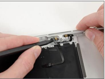
• Carefully pry the first microphone up off the upper case.
