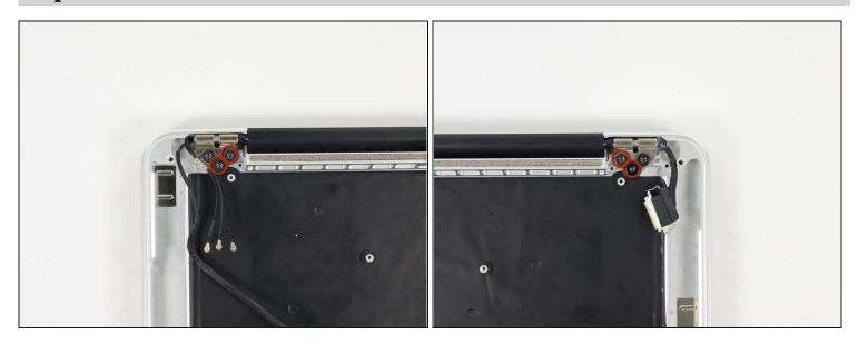
• Remove the four inner 5.3 mm T8 Torx screws (two on each side) securing the display to the upper case.
