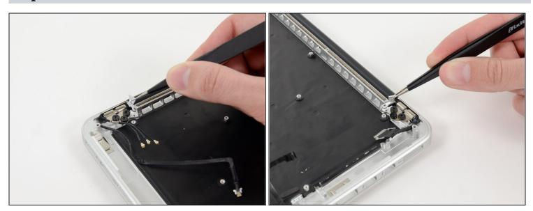
Use a pair of tweezers to lift aluminum hinge brackets off the right and left display hinges.
