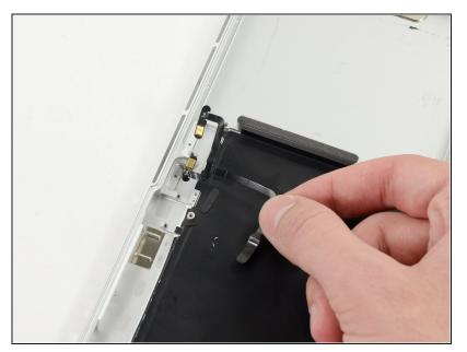
Lift and remove the microphone assembly out of the upper case.
