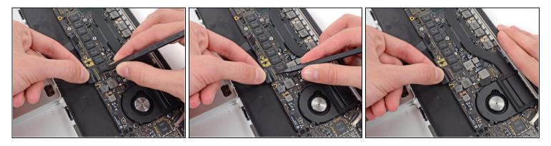
• Use the tip of a spudger to flip up the retaining flap on the keyboard ribbon cable ZIF socket.
