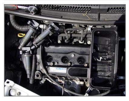
ignition coil connector and place them on a workbench (taking care to identify each coil), or leave the coils plugged in and stored to the left and above the engine.
