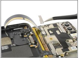
• Use a pair of tweezers to remove the small metal shield which covers the battery and the charging port and headphone jack flex cable connectors.
