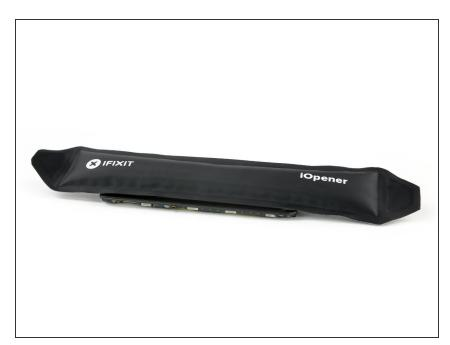
Apply a <u>heated iOpener</u> to the screen and all edges of the phone for at least two minutes, to loosen the adhesive.
