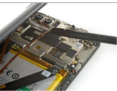
Use a spudger to pry up and disconnect the fingerprint flex cable.
