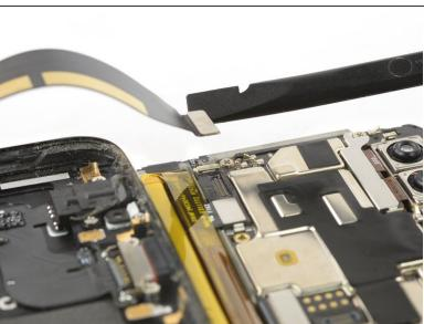
• Use a spudger to pry up and disconnect the charging port and headphone jack flex cable.
