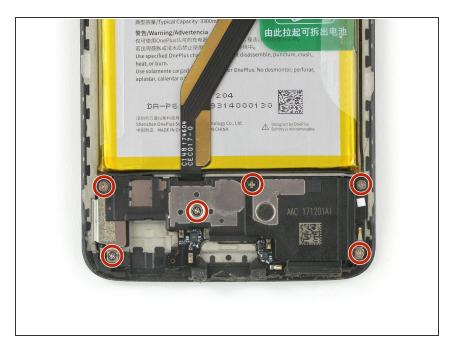
Remove the six Phillips #00 screws (2.9 mm length).
