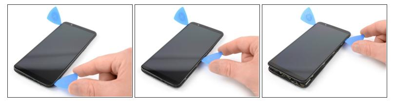
Slide the opening pick around the bottom right corner and then up along the right edge of the phone to open the plastic clamps that secure the backcover.
