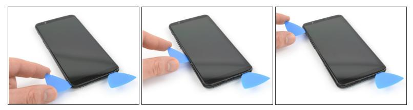
Slide the opening pick around the bottom left corner and then up along the left edge of the phone to open the plastic clamps that secure the backcover.
