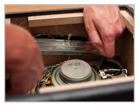
Glue the new reverb tank into place following the directions provided with the glue or epoxy of your choice.
