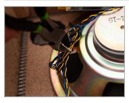
Use wire cutters to remove the zip tie fastening the wires to the speaker.
