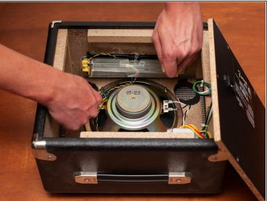
Saw the adhesive from in between the reverb tank and the cabinet until the reverb tank is released.
