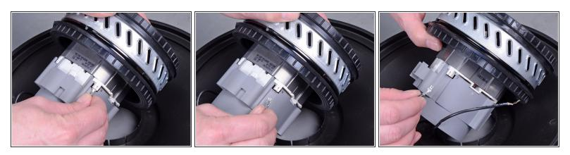
• Disconnect the two motor wires from the motor by pulling them straight out of their sockets.
