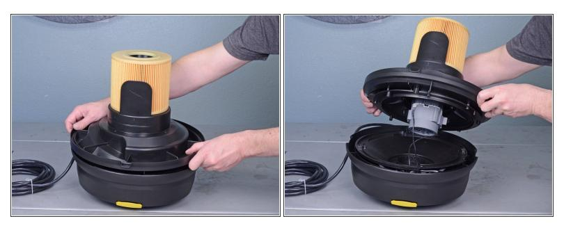
Carefully lift the motor/filter away from the housing until you can access the motor wires.
