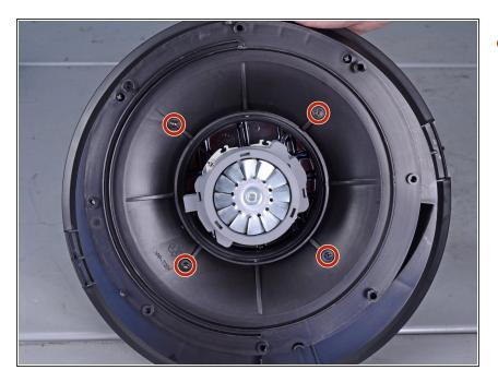
Remove the four T15 screws securing the motor flange.
