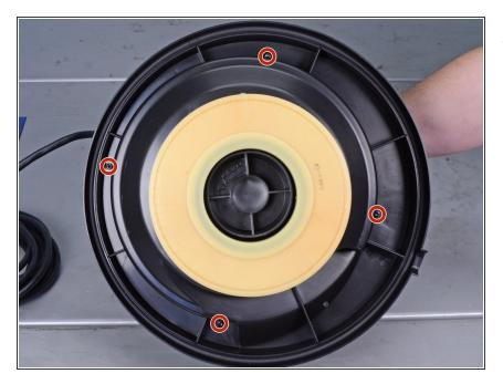
• Remove the four T15 screws securing the top assembly.
