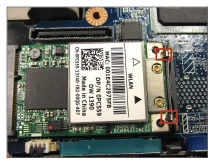
Push on the tabs indicated in the picture until the card pops up slightly then pull the card out at an angle.
