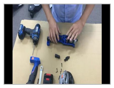
Adjust the position of the wiring. Reassemble the Immobiliser Trigger and then the Switch Button.
