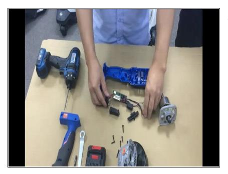
• Assemble the new Switch and electronic components.
