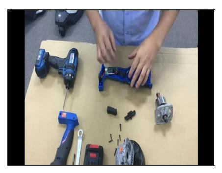
• Remove the faulty switch and the electronic part.
