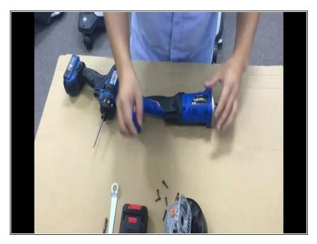
Remove the top case. Remove the Switch button, the Immobiliser Trigger and then the Engine.
