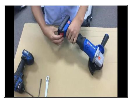
• Remove the battery and disassemble the Grinding Head.
