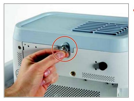
Turn the captive D-ring fastener on the bottom of the panel counterclockwise one-quarter turn and release.
