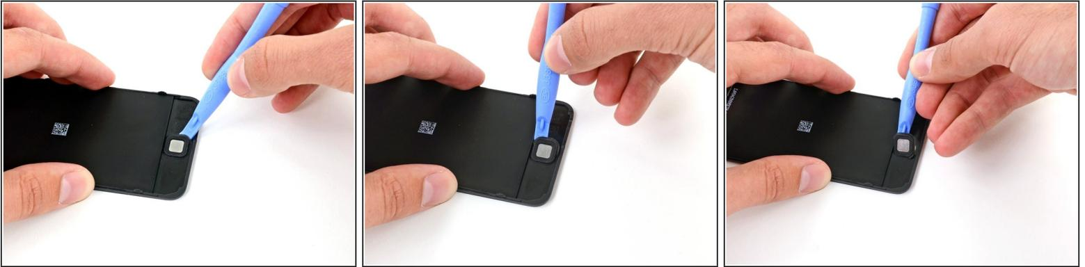
**i** Being careful not to rip any ribbon cables still connecting the two halves of the device, lay the display assembly flat so you can access the back of the home button.
