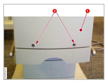
Remove the two screws (2) securing the front cover (1).
