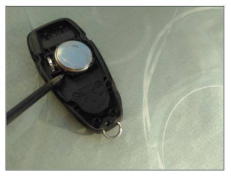
Remove the spent battery with the nonconductive spudger tool
