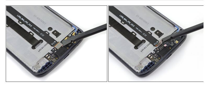
• Use a spudger to pry up and disconnect the daughterboard flex cable.
