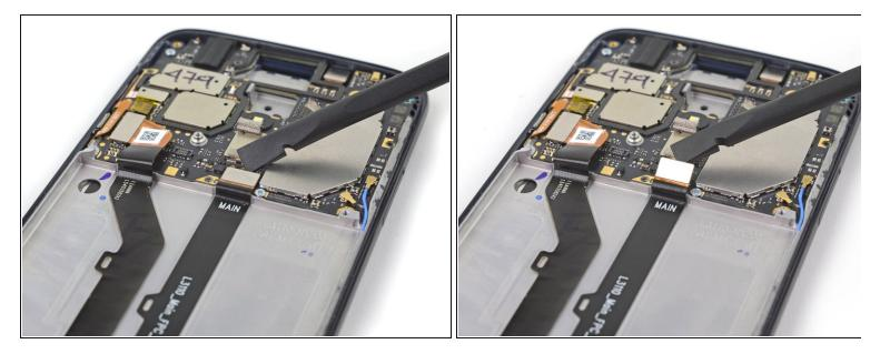
• Use a spudger to pry up and disconnect the daughterboard flex cable from the motherboard.
