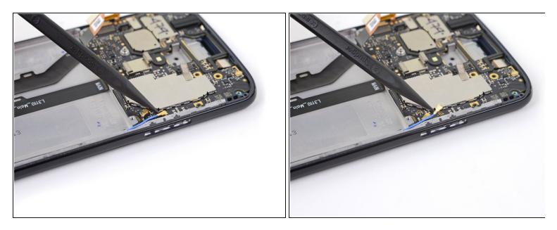
• Use the pointed end of a spudger to pry up and disconnect the blue antenna cable.
