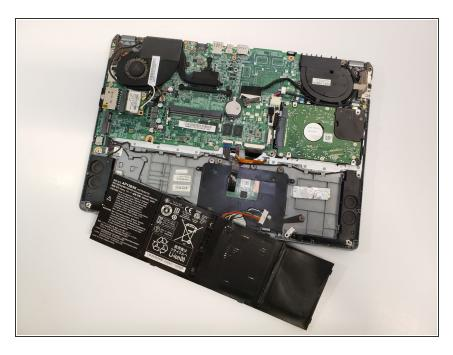
• Carefully take the battery out of the device.
