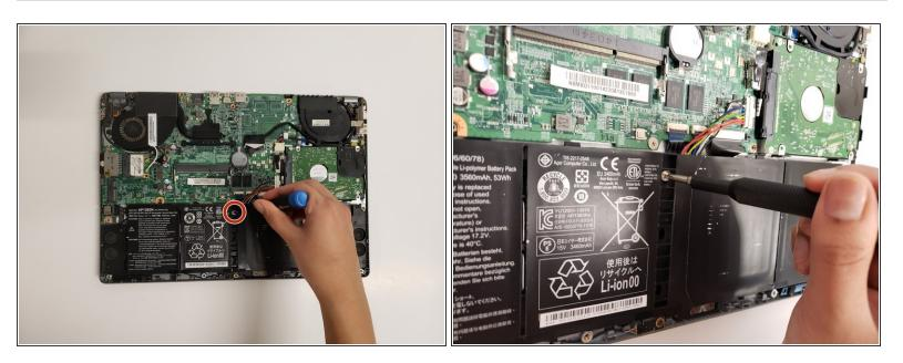
• Remove the Phillips #0 screw from the middle of the battery.
