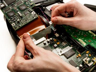
Pry out the DLP support piece by gently wiggling it side to side while applying a steady pull. It will slide out.
