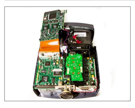
Remove the 2 remaining T10 Torx 8mm screws securing the motherboard to the power supply.
