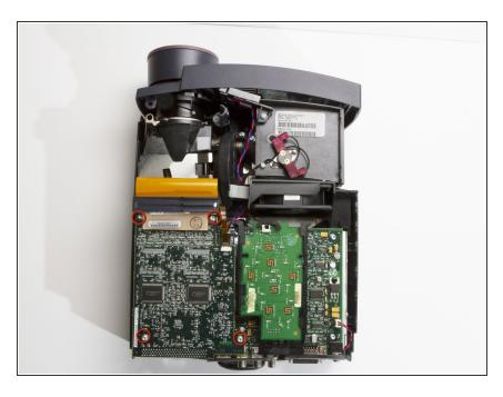
Remove the four T10 Torx 8.5 mm screws holding the DLP board in place.
