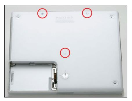
Remove the one 10 mm and two 20 mm hex screws using a 2mm hex.
