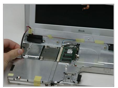
Lift the upper case off completely and disconnect the red and black speaker cable from the logic board.
