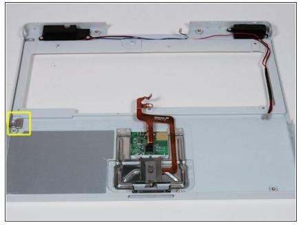
There is a magnet that allows the computer to detect when the laptop is closed. If this magnet is not present your computer will not automatically go to sleep. Be sure the magnet is in the position indicated.
