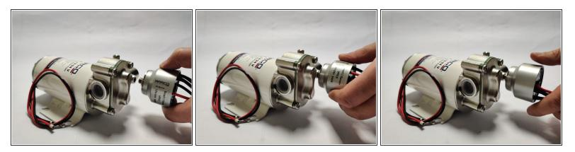
• Screw the new sensor by hand for the initial part.
