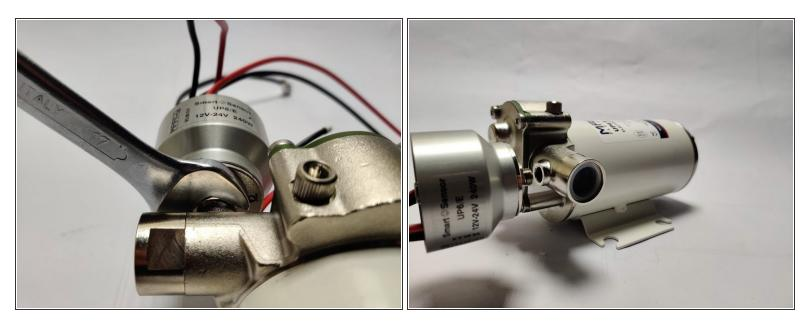
• Use the 17mm wrench to unscrew the sensor.
