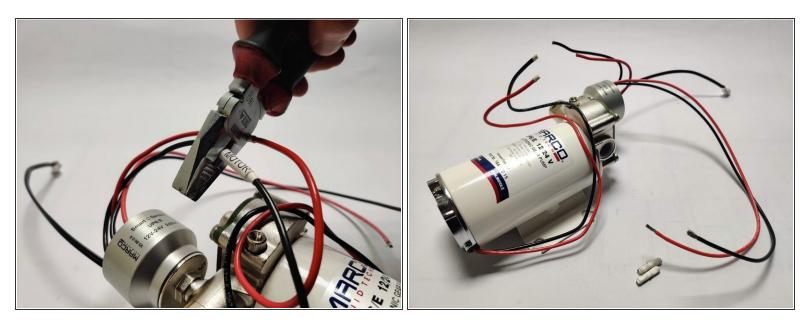
Use the pliers to cut the red and black cables before and after the joint.
