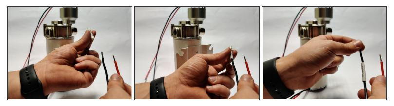
• Insert the heat shink tubing on both motor's cables.
