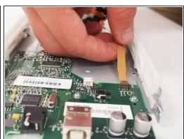
Use careful pressure to remove both cables from the PCB.
