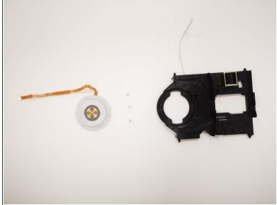
Using the T6 driver, remove the three screws surrounding the zip disk reader.
