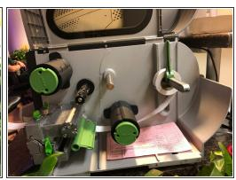
Open the machine by lifting the right side up.
