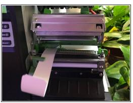
Weave the new armband strip under the back and green cylinder and through the press. Close the press by pushing it down firmly.
