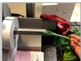
Slide the green bar to the right then pull it down to remove the roll of armbands.
