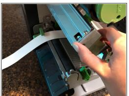
Assess where the problem is within the machine. Press the green button that says "push" to release the end of the armband that is clamped in the machine.
