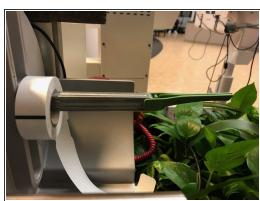
Replace the previous armband roll if it's damaged and insert a new roll by sliding it onto the device and pushing the green bar back into place.
