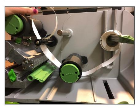
Remove the armband strip from under the press.
