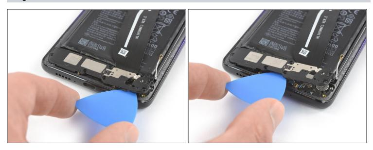
• Work your way along the bottom edge of the loudspeaker cover into the direction of the charging port. Use the opening pick to pry up the loudspeaker during this procedure.
