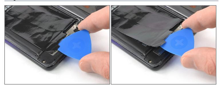
• Slide an opening pick under the bottom end of the black protective foil that covers the battery. Use the opening pick to loosen the adhesive that attaches the foil to the loudspeaker.
