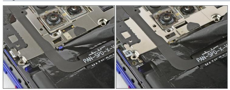
• Use the pointed end of a spudger to unhinge the motherboard cover from the small hook above the left side of the battery.
