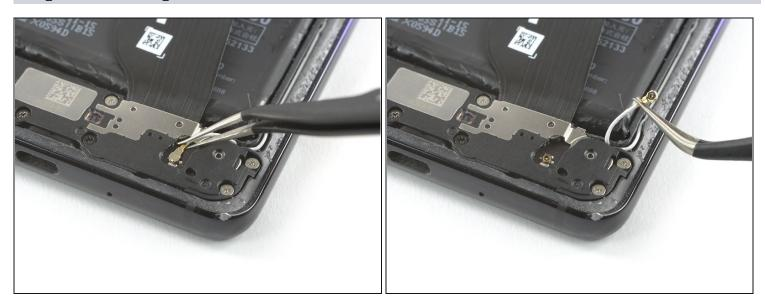
• Use a pair of <u>tweezers</u> to pry up and disconnect the antenna cable.
