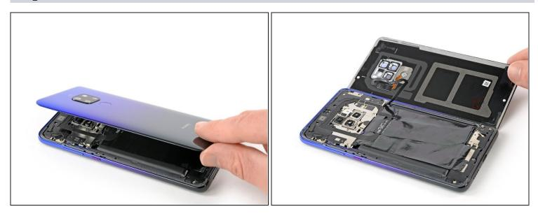
• Carefully fold the back cover to the right side of the phone assembly. Avoid tension to the fingerprint cable during this procedure.
