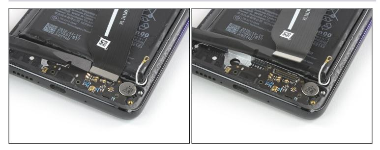
• Use a spudger to pry up and disconnect the connector on the bottom end of the main flex cable.
